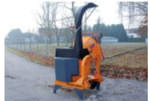
TVI 60 PT ; optional 270° turn able version for 3-point hitches
