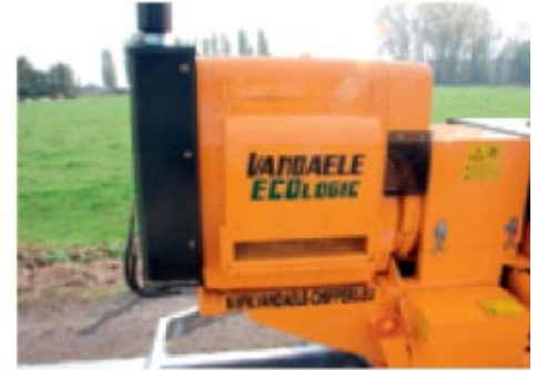
Standard Equipment: 52 HP HATZ diesel engine with "Silent Pack" on engine driven units.
