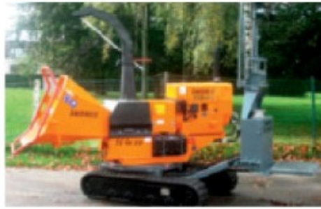
TV18-23 DTC EcoLogic; Hydraulic driven on a self propelled tracked undercarriage.
