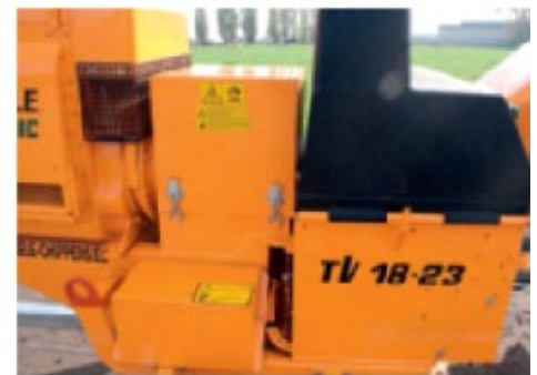
Diesel version: in-line mounting of the engine and chipper housing with direct drive system – no clutch or belt drive
