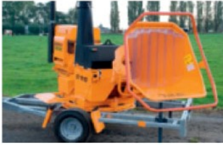
TV18-23 D EcoLogic; 360° turn able option on road trailer;
