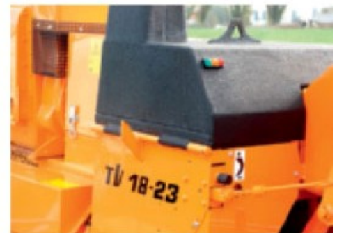
Standard noise reduction kit on the diesel version: extra noise dampening coating on the top cover, the infeed funnel and the coupler
