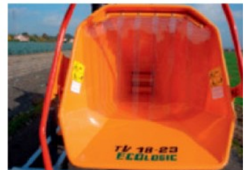
Transparent flaps in the infeed funnel come standard on diesel engine driven version. Increased operator safety and extra noise reduction.
