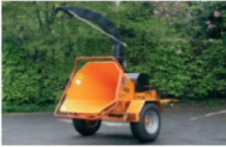
TV250 P; Tractor driven, mounted on a single axle slow transportation trailer (optional).
