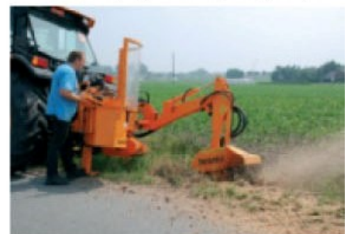
Optimum visibility on the job – the operator area is situated behind a Plexiglas screen.
