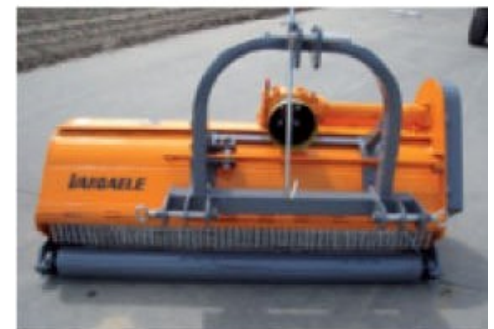
Height adjustable roll, mounted in the rear (optional).
