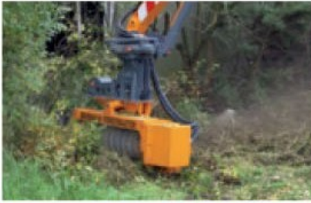
Hydraulic driven model to be attached to a crane arm or mowing arm.
