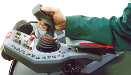
Single-lever Low Pressure mixed (elec. + hydr.) controls
