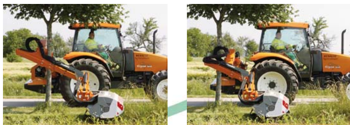
It is possible to mow round obstacles without changing course before and after the obstacle.
