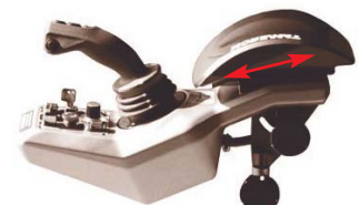
Single-lever electrical proportional controls
